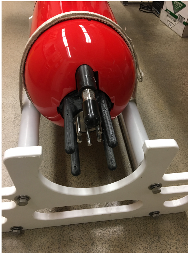
Figure 8: Velocimeter mounted on the nose of DG043, above the RSI MicroRider turbulence sensor.
